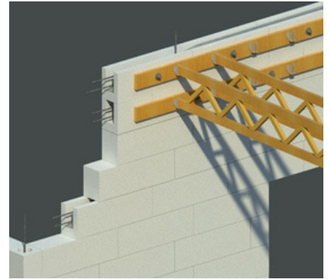
Fig. 23 B: Anchoring wood top plate to U-Block top bond beam.
