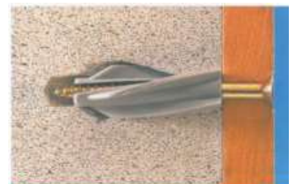
Fig 30: Minimum Screw Length
